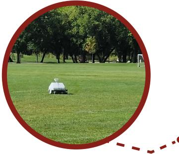
The Parks & Maintenance Department began using the Turf Tank robotic striper to paint athletic fields. Using this technology greatly reduces staff time and resources required to setup and stripe a field. In addition, the robot uses less paint than traditional striping methods, saving money each month.
